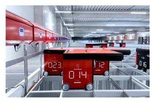
Rocket Solution develops innovative, standardized and highly space-efficient shuttle systems. These systems consist of high-dynamic storage vehicles that operate within the rack to provide and buffer bins and trays.
